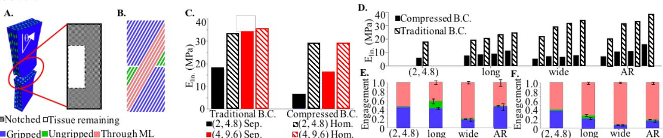
**Fig. 1** (A) Schematic of the separate model, with mid-length notch geometry. (B) Three fiber groups (same colors used in E & F). (C)  $E_{lin}$  of Hom. and Sep. models. (D)  $E_{lin}$  for Sep. models (dimensions increase from left to right within each group). Fiber engagement with (E) traditional and (F) compressed B.C.s.
