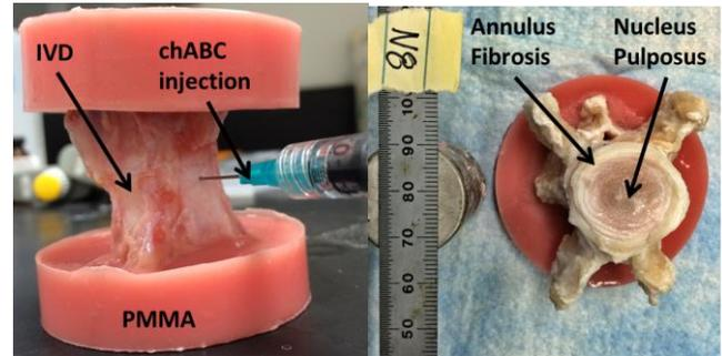
**Figure 1. (A) Potted motion segment sample with enzyme injection. (B) Cut disc sample with AF and NP visible.**
