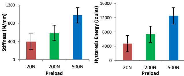
**Figure 2. (A) Linear relationship between average torsional stiffness and preload. (B) Linear relationship between average energy loss and preload.**
