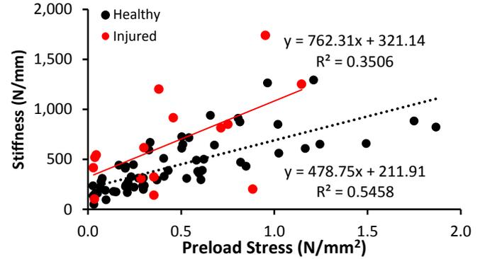
**Figure 3. Comparison of normalized torsional stiffness with respect to axial compressive stress for healthy and injured discs.**
