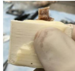
Figure 3: L5 bone with uniaxial cuts by a diamond saw while fixed into the 3D printed fixture
