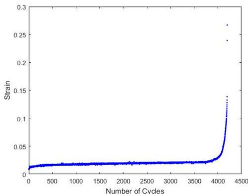
Figure 5: 722E L5 fatigue curve, showing strain vs. number of cycles
