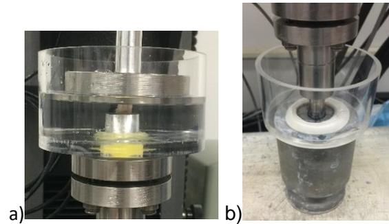
Figure 4: a) Instron machine set-up with loaded bone
