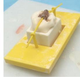
Figure 2: Excessive PMMA bubbling with an example of a loaded bone into the fixture
