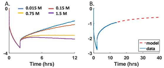
**Figure 3:** A) Disc height recovery for each osmotic loading group (PBS solution). B) A representative sample of data and model fit.
