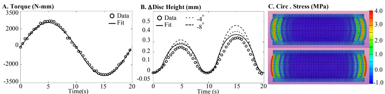
Fig.1 (A) Torque with  $\pm 5^\circ$  axial rotation. (B) Change in disc height change (small peak for  $+5^\circ$  and big peak for  $-5^\circ$ ) with rotation for data and FEM predictions (e.g., fiber angle rotation of  $4^\circ$  and  $8^\circ$  towards the horizontal plane). (C) Circumferential stress at  $+5^\circ$  (top) and  $-5^\circ$  (bottom).
