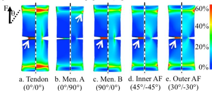
**Figure 2: Strain map (front | back) at predicted failure initiation. Arrows indicate maximum local strains.**
