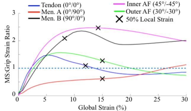
**Figure 3: MS:grip ratio versus global strain for four fiber architectures (all Notched). X denotes predicted failure.**
