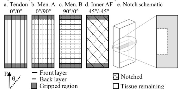
**Figure 1: (a - d) Schematic front view of specimens showing fiber architectures and (e) schematic of notched geometry.**
