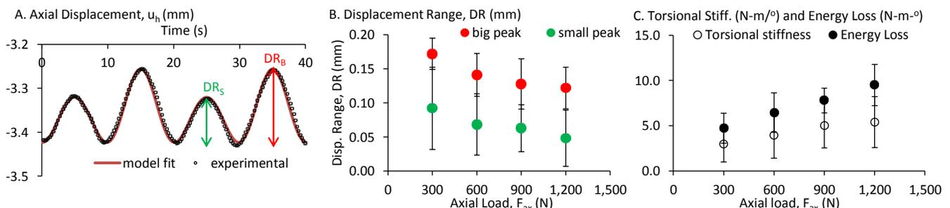
Fig 1. A) Axial displacement during torsional loading, B) Displacement range for both peaks and C) Torsional stiffness and energy loss ( $p < 0.001$  for all).
