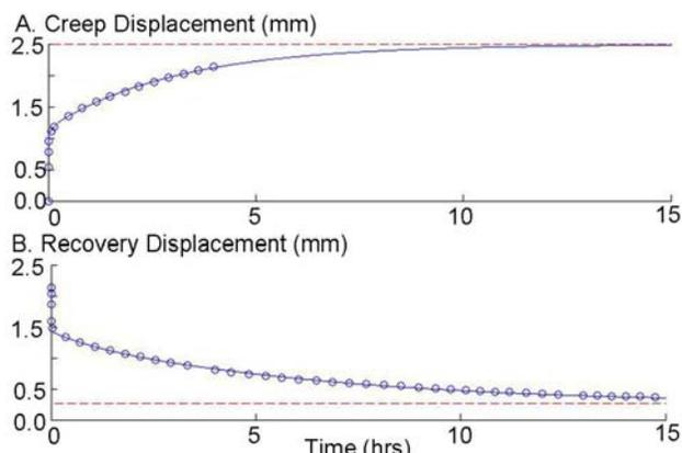
**Fig 1:** Representative figure of the A) Creep & B) Recovery behavior. Equilibrium displacement and experimental data (not all data points shown) is denoted by the dotted red line and circles, respectively.
