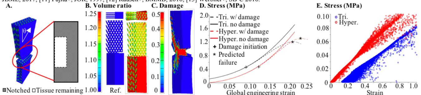
**Fig. 1** (A) Schematic of the separate AF model in tension (blue: matrix; green: fibers). *Zoomed:* mid-length notch geometry. (B) Tissue relative volume with free-swelling (Ref.: reference configuration). (C) Tissue failure in tension. (D) Stress-strain response (Tri: triphasic; Hyper: hyperelastic; dashed lines of lighter colors: predicted damage curves). (E) Stress-strain response of the extracellular matrix under uniaxial tension.
