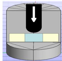
**Figure 1.** Schematic of confined compression apparatus used to load half-cylinder agarose samples (light blue) in cartilage (yellow boxes). The diameter of the indenter (black piece) was equivalent to the diameter of the construct. The front face was flat to acquire images for strain analysis.
