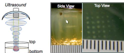
Figure 1. Schematic of HMIFU application. Gel phantom showing rasterized pattern of denaturation (Study A). (scale: 1 mm)
