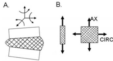
**Fig 1:** (A) Schematic showing *in situ* AF boundary conditions and multi-directional loading, (B) Uniaxial and biaxial sample geometry and loading
