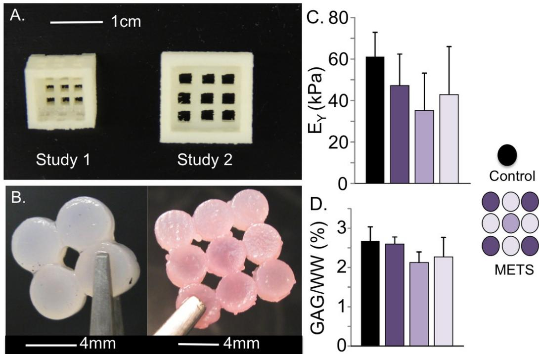
**Figure.** A) 3D printed porous molds. B) 2x2 and 3x3 METS samples. C) Compressive Young's modulus and D) glycosaminoglycan content of individual controls (black bars) and various regions in the METS (purple). No differences were observed with respect to the control.
