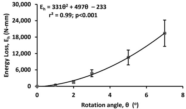
**Figure 2:** Energy loss with rotation angle.
